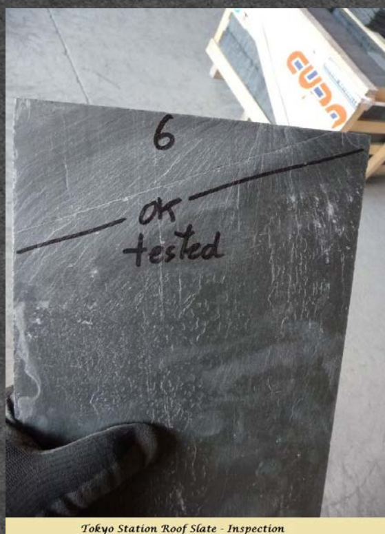
Tokyo Station Roof Slate - Inspection
